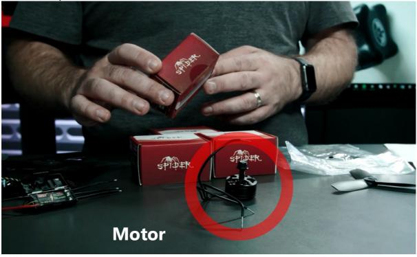
The motors supply the power for the drone to move.
