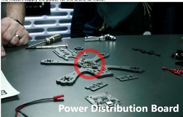
The electronic speed controllers, motors etc mount into the power distribution board.
