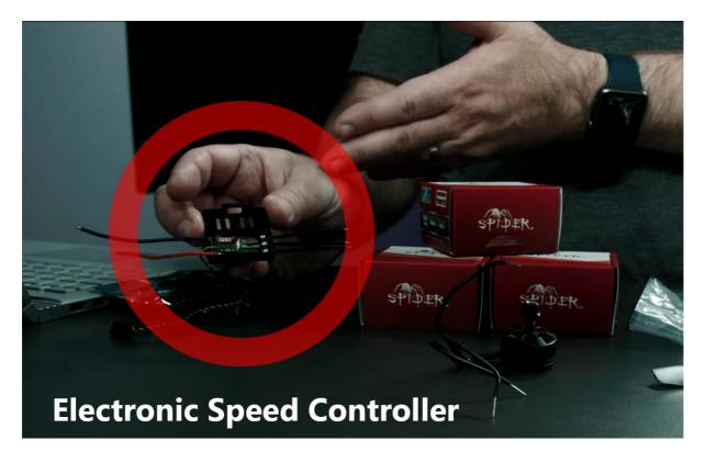
Electronic Speed Controllers control the signal that goes to the motors and tells the motors how fast to spin.
