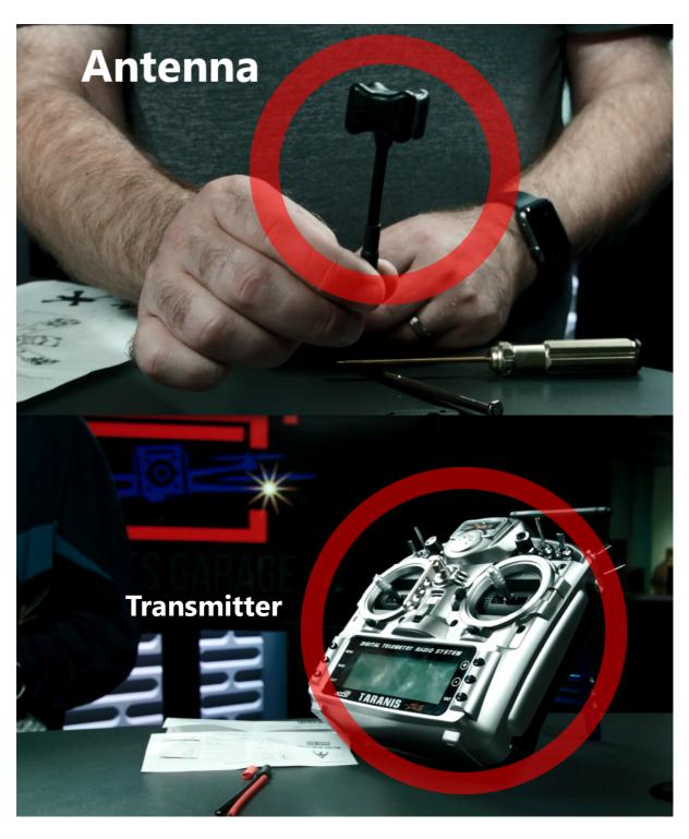
The camera hooks to the video transmitter which has an antenna which transmits the video to the pilot who is flying the copter.
