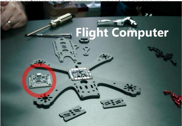
The flight computer along with the motors allow the drone to fly.
